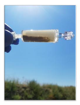
9) After filtration, the inlet and outlet of filters are capped at each end, labelled with location ID and volume filtered, placed into a sterile secondary container (Ziploc), sealed, and immediately placed in a cooler. Filter is considered self-contained at this point.
